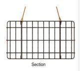
Plan view of a typical pad foundation cage up to 3m long, 3m wide or 2000kg
