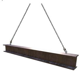
Structural steelwork and fabricated steel assemblies shall have designed lifting points or a method for making a positive connection to a removable lifting bracket.
