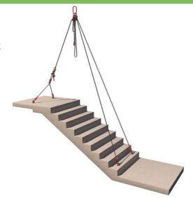
Example opposite shows a lever hoist being used on the 'upper' section of stairs to aid configuring the stairs into an 'install' orientation.
