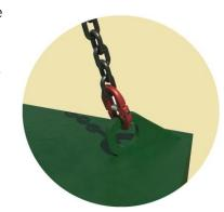
Check attachment points for the chain/wire rope slings for any signs of deformation that could impede the safe use of the suspended personnel carrier.
