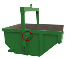
VII. When the bale arm is lowered, ensure the catch does not engage so that the centre of gravity ensures that the skip will then lift in the tipping position.
